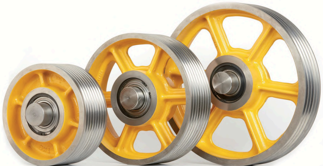
PULLEY: GREY CAST IRON GG26 / HARDNESS 190 - 230 HB / SHAFT: C35-C45-42CrMo4
